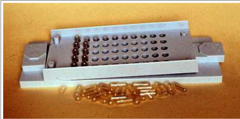
Figure 3.11: A small and cheap device for manually filling small quantities of hard gelatin capsules. With the top piece raised, as on the right, the pollen is brushed into the capsules. Once the top piece is lowered, as on the left side, the capsules can be closed.
