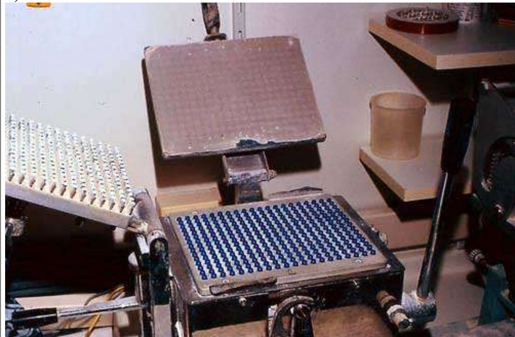
Figure 3.10: Medium-size hand-operated capsule filler. a) One machine separates the capsule halves, sorts and places them into separate trays. b) A second machine allows filling of capsule halves in presorted trays from a) and then closes the capsules. Using both machines, 1500-4 000 capsules can be filled, compacted and closed per hour by one person.
