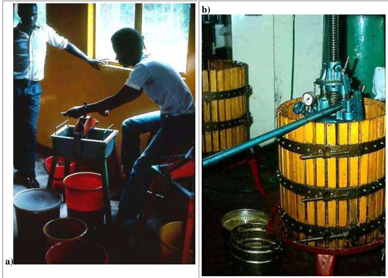
Figure 2.9: a) Small, common honey press in Zambia; b) Larger honey press used to squeeze honey from cappings in Italy.
