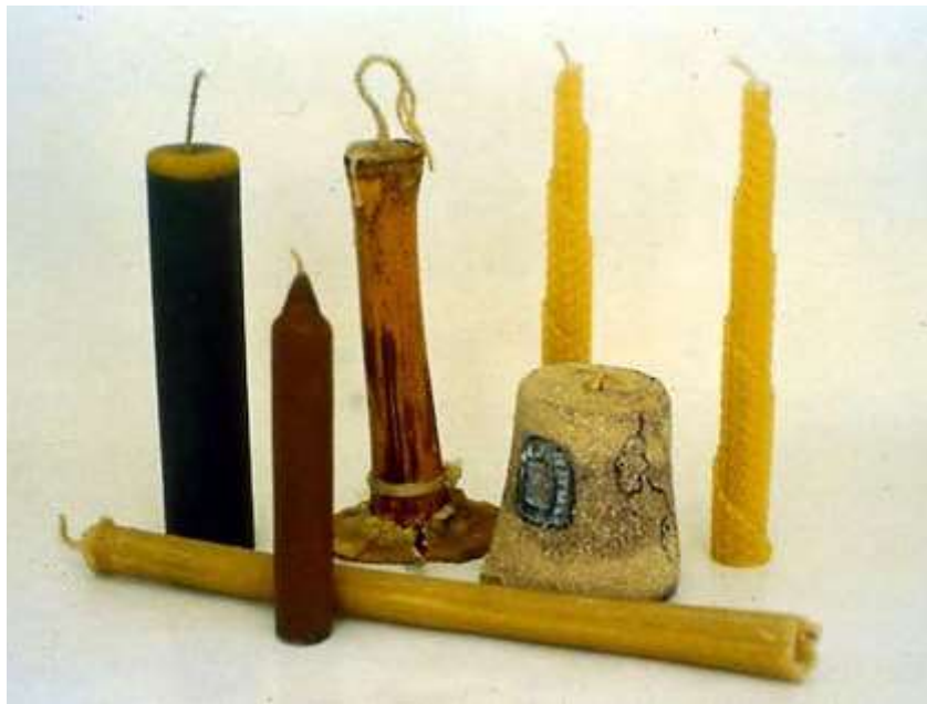
Figure 4.7 : A display of homemade candles from West Africa (from left to right): stained candle moulded in PVC pipe, coloured wax with trimmed tip, candle still inside of bamboo mould, 2 candles rolled from wax foundation sheets, decorated candle from plastic cup mould, candle from bamboo mould (bottom).
